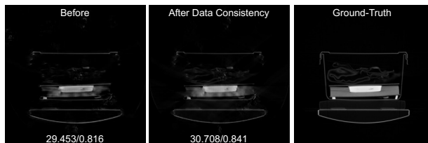
Figure 3: One of the predicted images from the inference model and its final image after the data consistency-based refinement with our projector. The PSNR/SSIM values are indicated at the bottom.
