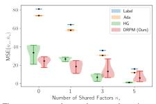
Figure 3. The mean squared errors between the estimated number of shared factors  $\hat{n}_s$  and the true number of shared factors  $n_s$  across five seeds for the Label-VAE, Ada-VAE, HG-VAE, and DRPM-VAE.
