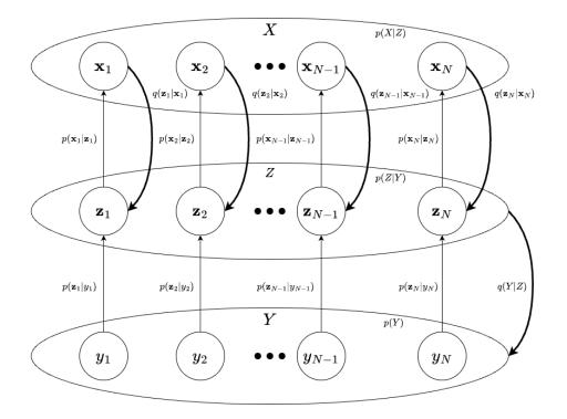
Figure 9. Generative model of the DRPM clustering model. Generative paths are marked with thin arrows, whereas inference is in bold.
