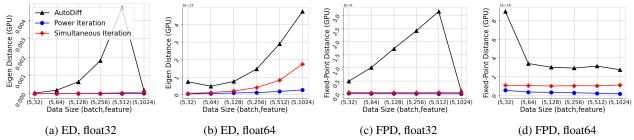
Figure 5. Symmetric A sampled from Gaussian distribution with activation, precision evaluation with eigen distance and FPD.
