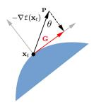
Figure 3. Descent direction projected onto a Riemannian manifold for the sphere constraints.  $-\nabla f(\mathbf{x}_t)$  is the PGD direction,  $\mathbf{G} = Proj_{\text{RM}}(-\nabla f(\mathbf{x}_t))$  is the descent direction on the Riemannian manifold, and  $\mathbf{x}_t$  is on the Riemannian manifold.
