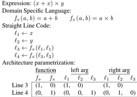
Figure 4. Symbolic expressions are built from operators in a Domain Specific Language and represented as straightline code. Each line of code is parametrized by three one-hot binary vectors specifying a function from the Domain Specific Language, and left/right arguments from earlier lines. (The first lines of code simply load variables into scope.) The bottommost box shows the 6 one-hot vectors encoding the example expression ( $\alpha$  in the paper).
